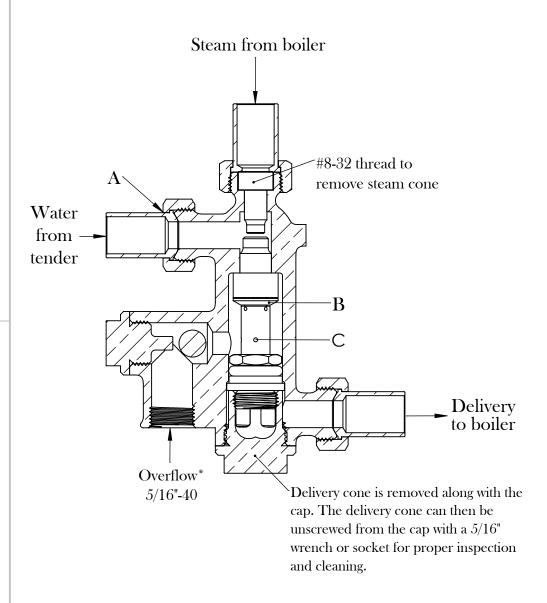
\*It is important to note that if water is visible from the overflow during operation, the injector is not properly delivering water. Opening or restricting the water valve will help the injector to run "dry." A water valve with fine adjustment, such as a needle valve, is strongly recommended.
