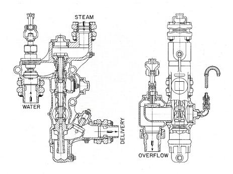
The prototype 1918A Injector, cross sectional view.
