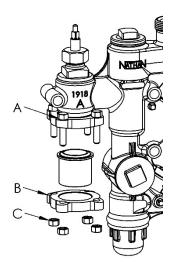
The compressing flange (B) must be placed over your tubing before soldering on the connection!!! Note that there are reliefs on one side the flanges (Fig. B). These must face inward toward each other. The nuts and bolts should not be clamping down on these chamfered edges.
