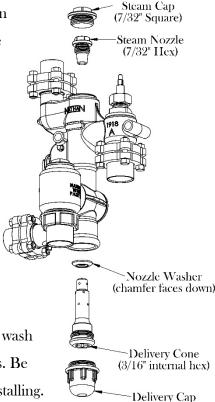
Do not remove the combining cone unless you are replacing it! Removal will damage it.
